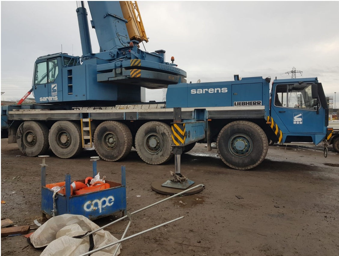
Equipment: Liebherr LTM1150-5.1 (2348) LOCATION: UK
