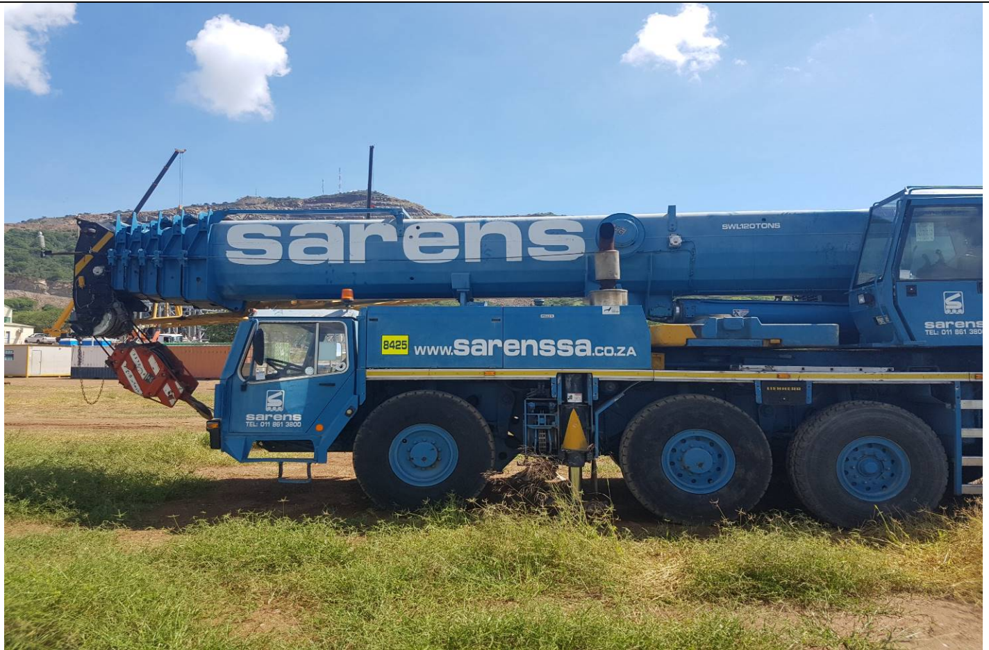
Equipment: LIEBHERR LTM1120 – K8425 LOCATION: South Africa
